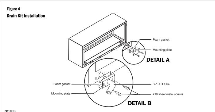
The large flange on the mounting plate is positioned at the bottom of the sleeve facing toward the sleeve. The drain tube must be rotated to a horizontal position to allow for the wall sleeve to be installed into the wall. Once the wall sleeve is installed, return the drain tube to a downward angle.
